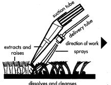
(T) Place the spray-extraction carpet shampoo nozzle on the carpet in a corner of the room. Press the control trigger (40) on the handgrip (11) until cleaning solution sprays onto the carpet. Then slowly draw back the upright nozzle in a straight line over the carpet.
